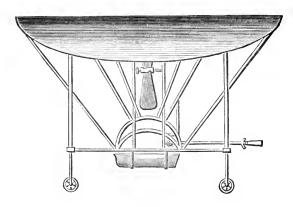
The balloon is made in an elongated form and having a membrane within same, below which latter air can be forced to keep the balloon always distended. The network is made of flat silk bands, which are placed longitudinally and transversely, and also diagonally if required. A single strong band attaches the net to the horizontal circumference of the balloon, which, in case of accident, would allow the lower membranes to rise and fill like a parachute.
